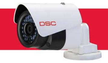
The DSC-B114-40 & DSC-B114-60 are IR Mini Bullet Cameras with a rich feature set that makes them ideal for applications that require high definition images and versatile performance even in challenging light conditions.
